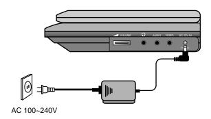
Note: When charging the battery pack, the charge light turns red and when the charging is complete, the light will turn green.
